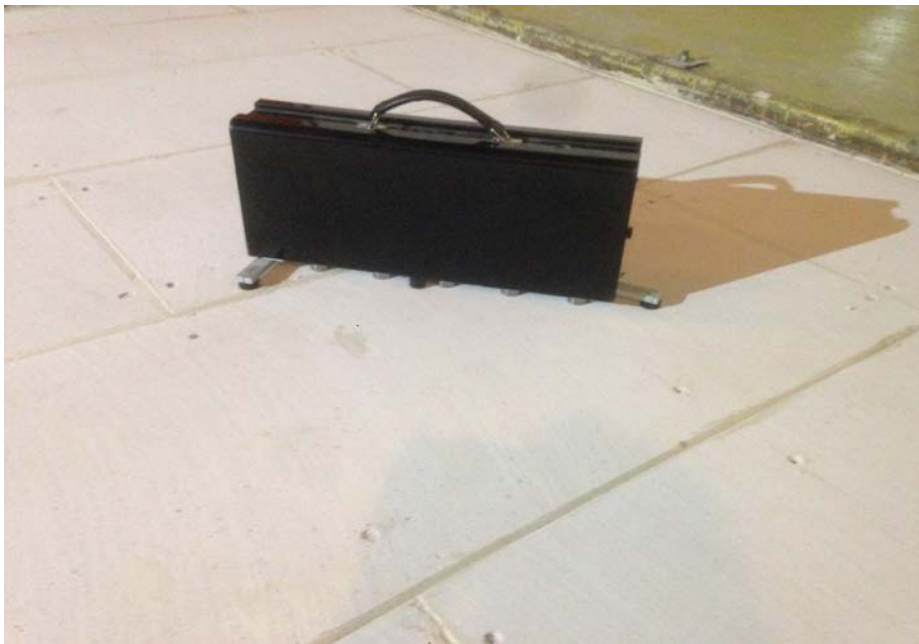
Figure 4: Tapping machine placed on panels showing screw-fixings
