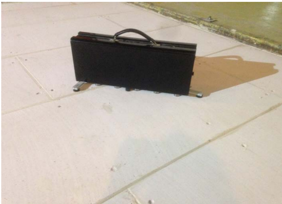
Figure 4: Tapping machine placed on floor panels
