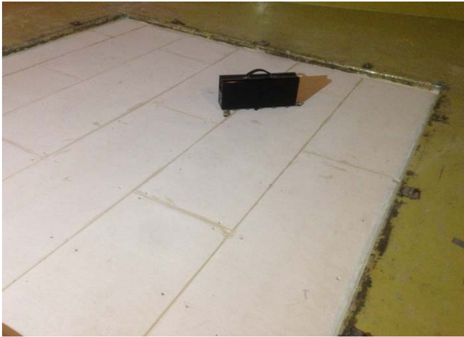
Figure 3: One of the tapping machine positions on the test floor
